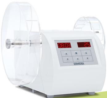
The TAR series is a USP/EP/JP compliant ERWEKA unit for testing friability and abrasion.
