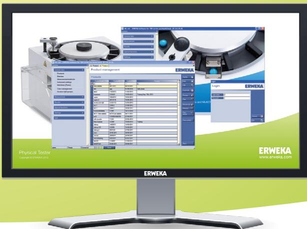
With the optional MC.NET software the TBH 325 can be controlled via a PC\*.
